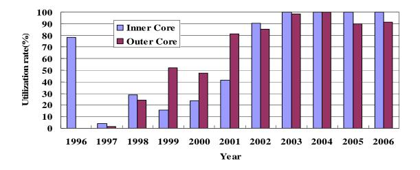
FIG. 3. The ratios of the occupied days of the irradiation holes to reactor operation days
